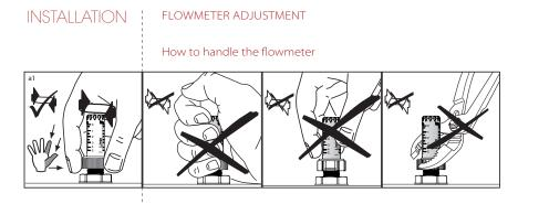
How to adjust the flow rate
