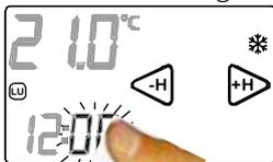
**MINUTES:** Keep the touch area of the MINUTES pressed and set the minutes using the keys ◀ ▶ (Fig. 17).
