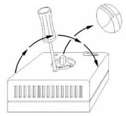
In order to don't damage the switch is recommended to remove the cover following the direction indicated by the arrow.
