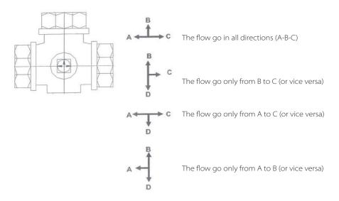
L valve operation: with the handle disassembled is visible, on the stem, a L mark, which indicates the running direction of the ball's holes, allowing the following combinations:
